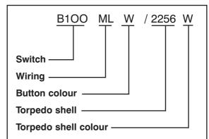
Example above: B1OOMLW/2256W is a single pole push button switch, push on / push off action, standard ML wiring, with a white push button. It is supplied with white torpedo shells and screws.
