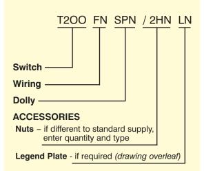
Example above: T2OOFNSPN/2HNLN is a toggle switch, double pole, single throw, with Faston connections and a short pear dolly that is nickel plated. It will be supplied with two hexagon nuts (not the standard one hexagon and one knurled nut) and a nickel plated legend plate.
