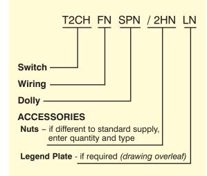
Example above: T2CHFNSPN/2HNLN is a toggle switch, double pole, double throw, with Faston connections and a short pear dolly that is nickel plated. It will be supplied with two hexagon nuts (not the standard one hexagon and one knurled nut) and a nickel plated legend plate.
