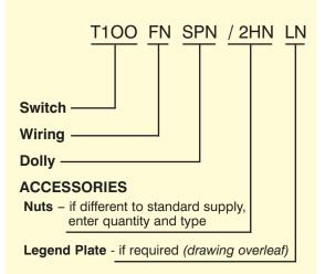
Example above: T1OOFNSPN/2HNLN is a toggle switch, single pole, single throw, with Faston connections and a short pear dolly that is nickel plated. It will be supplied with two hexagon nuts (not the standard one hexagon and one knurled nut) and a nickel plated legend plate.
